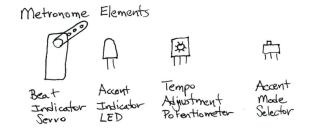
The key physical elements of the metronome demo: a servo used as a beat indicator, an LED to indicate accents, a potentiometer to set tempo, and a switch to select a 1/3 or 1/4 accent ratio.
