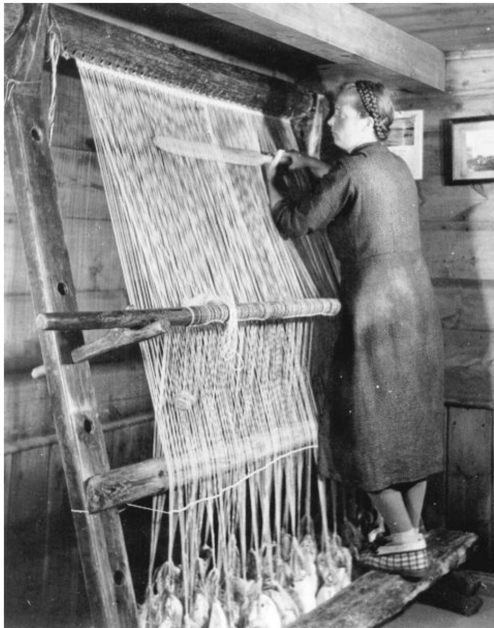
Swedish warp weighted loom used in rural regions up until as late as 1960s
