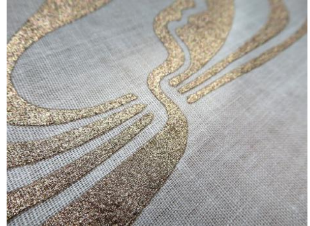
conductive ink (drawing/printing)
