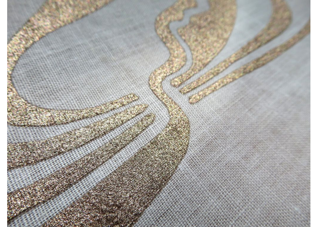
conductive ink (drawing/printing)
