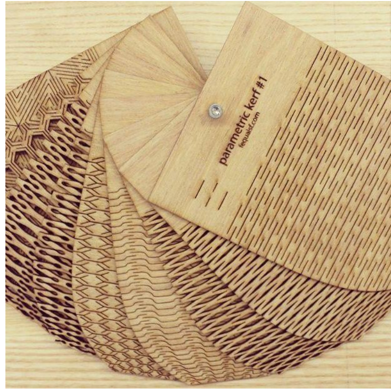
Laser cut wood - flexible in two directions, like fabric
