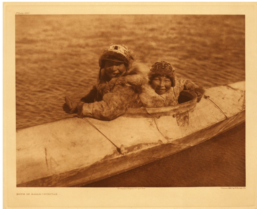
Kayak, Nunivak, Alaska, 1930 made from driftwood, seal skin and seal sinew
