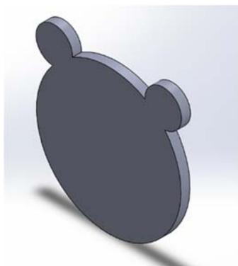
Go back to the front view. Now, we will make the eyes. Since they are cut out from the part, we'll use **Extruded Cut**. We will also draw on the top face and cut into the part
