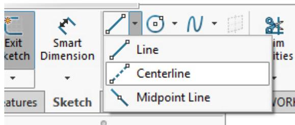
Draw a centerline straight up from the origin for about 1.5 inches. Check the **Vertical** Orientation in the left-hand panel to be sure your line goes straight up.
