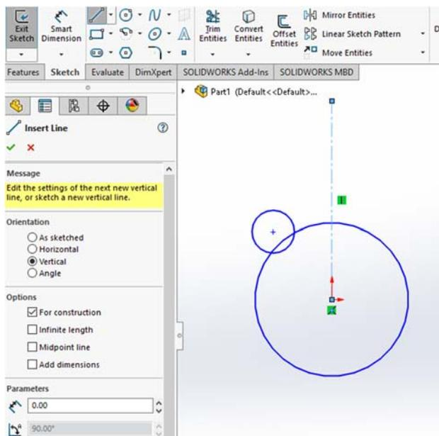
Notice the line property: **For construction** is checked; it is indicated visually as a dashed line. Click the green checkmark or press Escape to exit.
