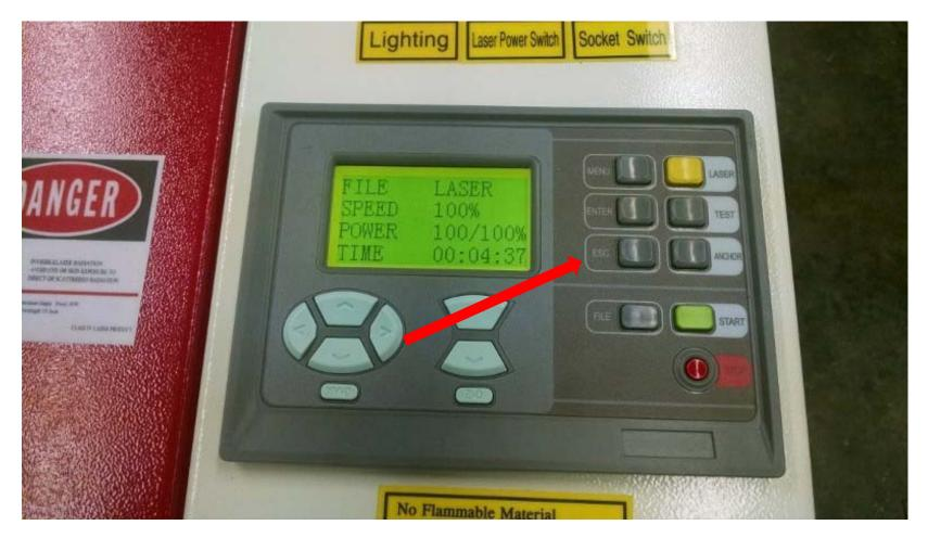
The laser cutter control panel has two modes. Press the Escape button on the control panel (not the computer keyboard) to switch modes.
