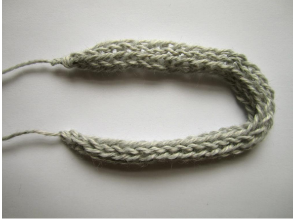
Knit / Crochet stretch sensor
