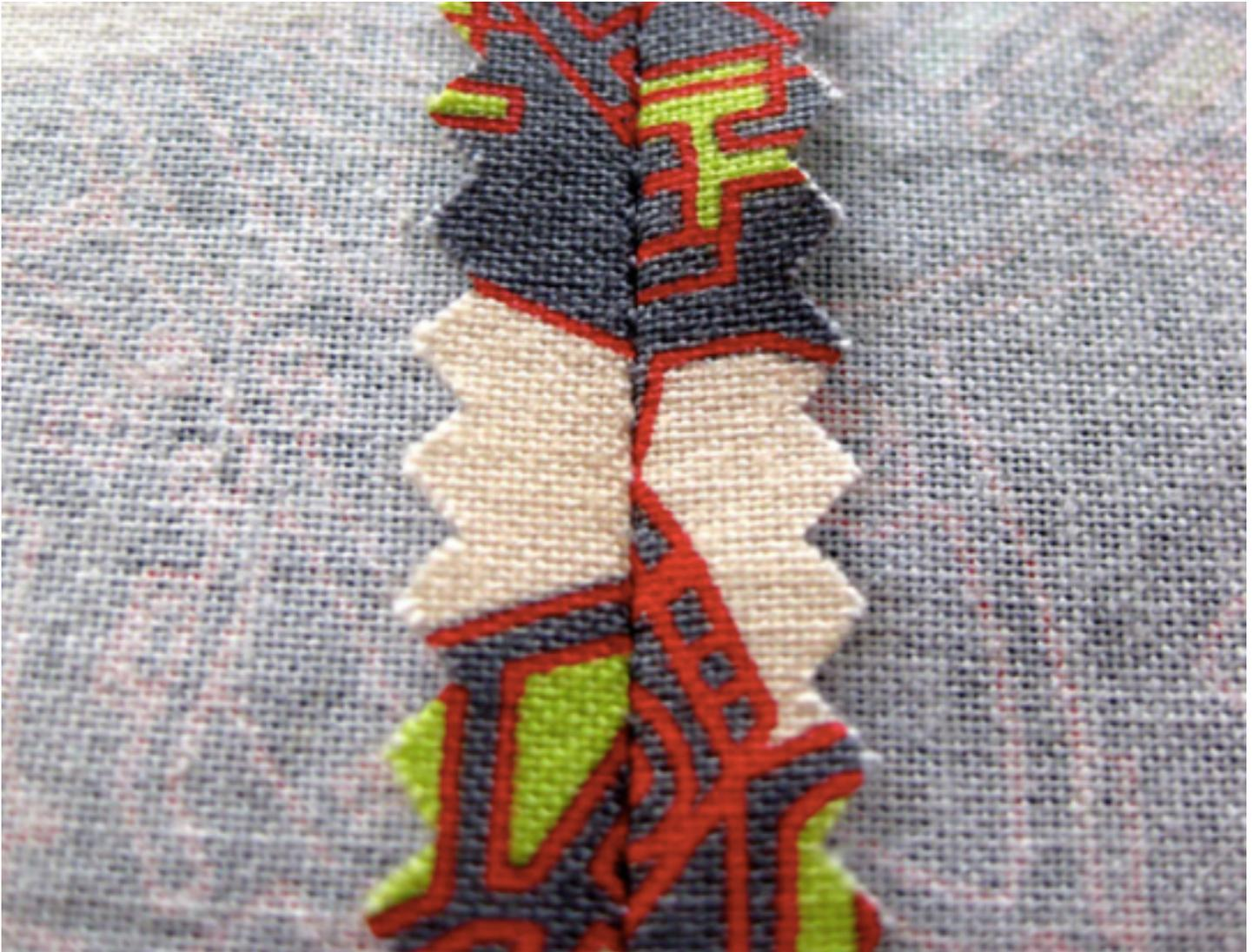
Pinking shears look like regular scissors, but instead of flat blades, there are little triangle "teeth" on the blades that make zigzag points in the fabric. Most woven fabrics are well suited for being cut with pinking shears, but some synthetic blends, silks, and thinner fabrics can sometimes bunch up and not give you a clean cut. If you've ever bought vintage clothes, you likely have come across a garment with pinked insides!
