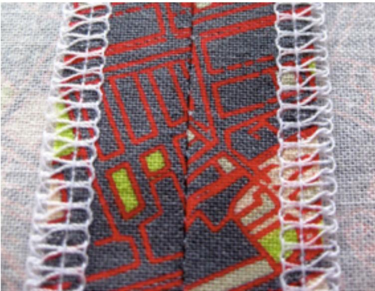
There are three main ways to use a serger for finishing a seam. First, pictured to the left, is much like the pinking shears option, where the seam is sewn and then the raw edges are finished individually by sewing along the edge with the serger machine.
