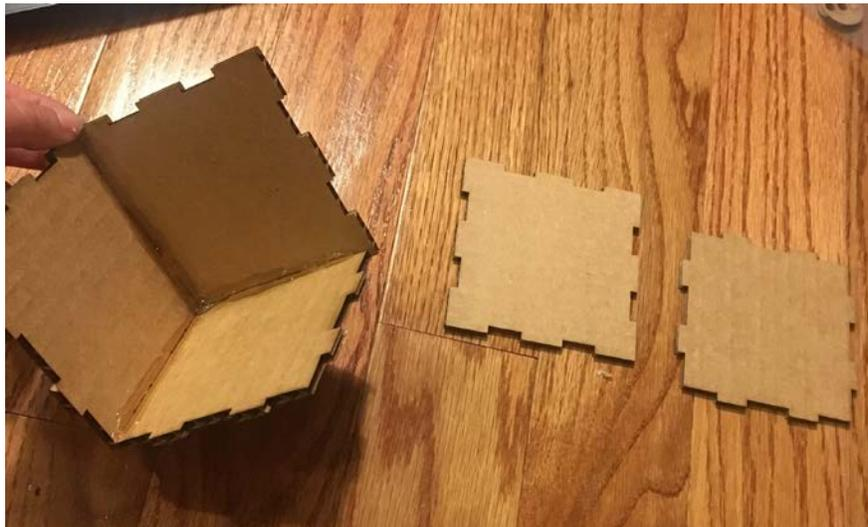
To make the guide for the crank, glue two E pieces together.
