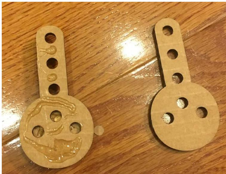
Glue the circles to the driver. The final assembly is 4 layers thick. Note that the hole in the circles does not line up with any of the holes in the driver.
